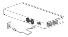
Figure 2-2-1 Connecting to the power
